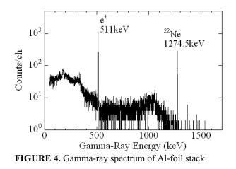
The three-dimensional distribution of the implanted <sup>22</sup>Na was evaluated with  $\gamma$ -ray measurements of the layers of the Al-foil stack. The  $\gamma$ -ray distribution on each of the foils was taken by an imaging plate to visualize the two-dimensional beam-spot profile at different depths. The distribution was found to be somewhat uneven, so the machine-parts sample was continuously rotated in the beam spot during implantation to average the distribution.
