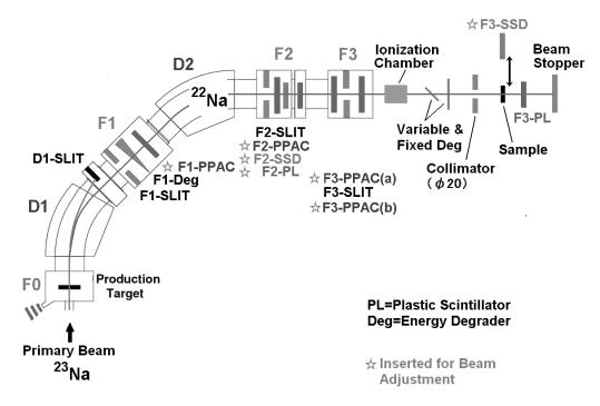
FIGURE 3. Setup of RIPS for RI-beam implantation.
