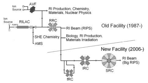
FIGURE 2. Conceptual diagram of the RIBF accelerators.
